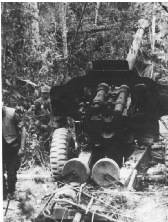
Marine Corps Historical Collection One of the 12 captured North Vietnamese Army 122mm field guns. With a range of 14 miles, it was the largest enemy artillery piece captured in Vietnam.
