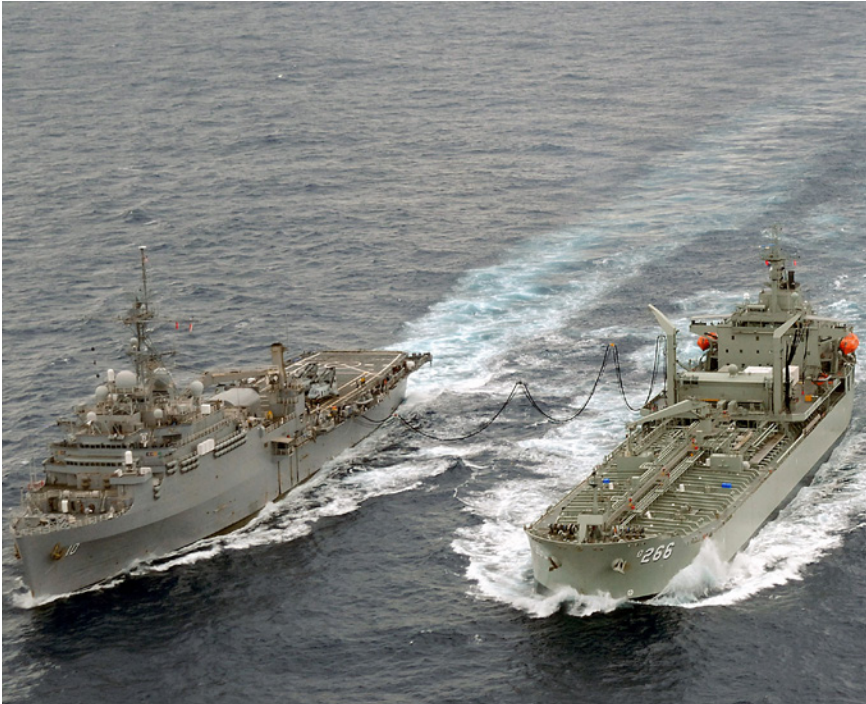
Figure 6. Ships of the TSP fleet equipped with consolidated replenishment stations can refuel U.S. Navy oilers at sea, thus enabling the oilers to remain on station with deployed fleet forces
