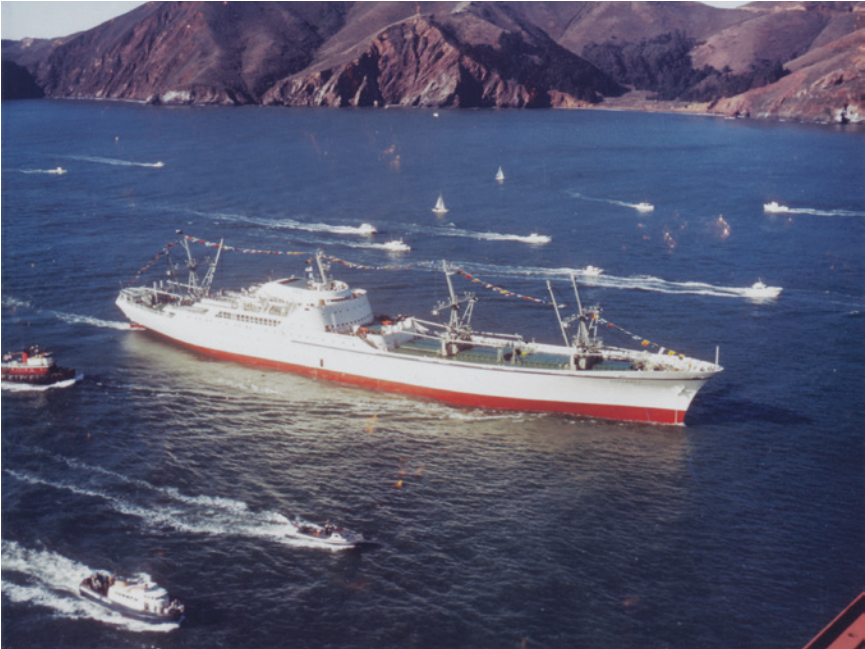
Figure 2. NS Savannah . The project was completely civil and was executed by Westinghouse. Savannah was a 21,800-ton ship with a cargo capacity of 10,000 tons and 60 passengers
