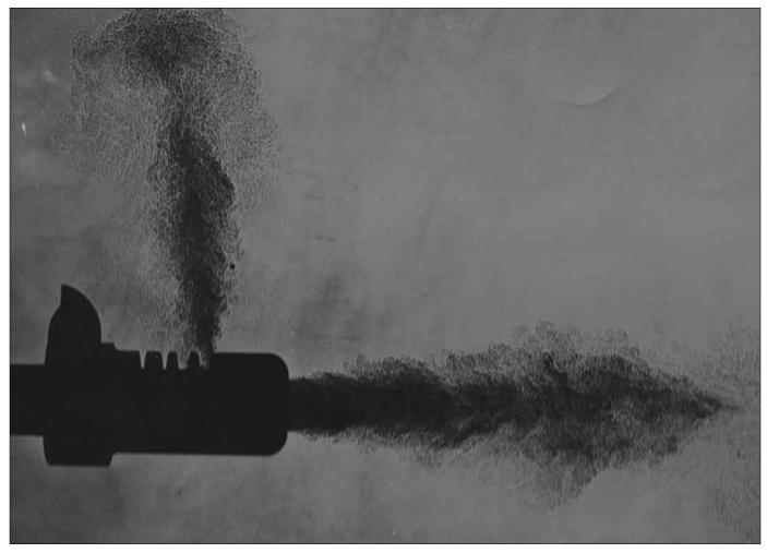
Cutts Collection, box 30, Historical Resources Branch, Marine Corps History Division Taken by spark photography, this image shows gas escaping through the ventilating ports on the top of the compensator.
