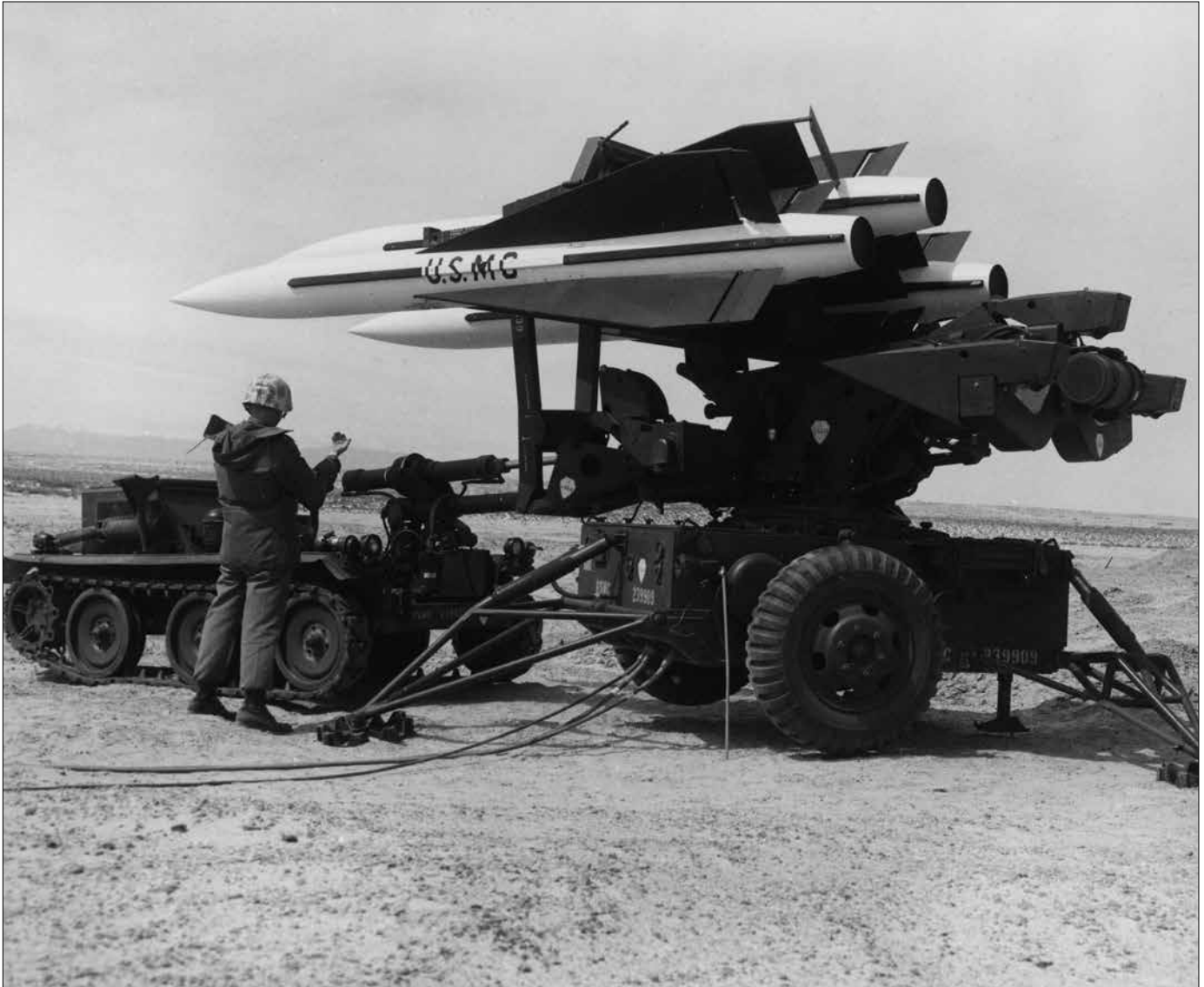
Official U.S. Marine Corps photo, by SSgt L. A. Pope, Archives, Marine Corps History Division, Quantico, VA A Marine Hawk crew loads three missiles onto a launcher using a tracked loader-transporter at Twentynine Palms in 1961.
