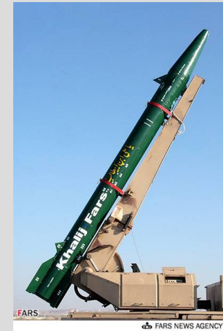
Fatah 110 anti ship version "Khalij Fars" Range: C. 200 Km. Terminal Guidance
