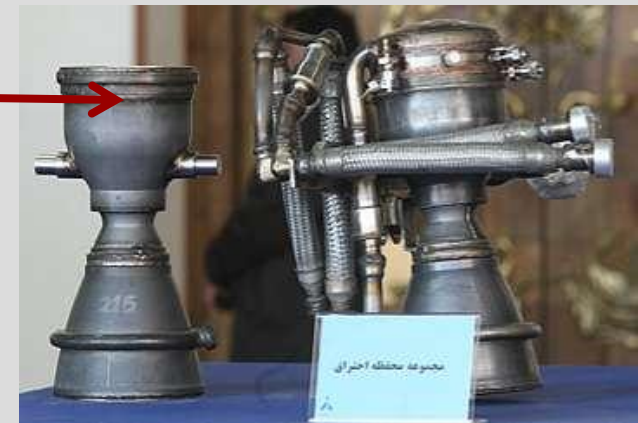
Gimbaled steering rocket motor Displayed in Teheran, Feb 3 2010
