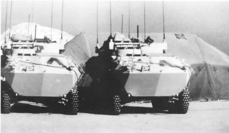
Two command and control variants of the light armored vehicle (LAV-C2) appear outside a command post in northeastern Saudi Arabia during Operation Desert Storm. The LAV-C2 was used as a mobile command post by LtGen Boomer and his subordinate division commanders during the war.
