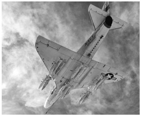
Underside of A-4 with multiple carriage bomb racks (MCBR) during first test flight, flown by the racks' developer, Captain William Fitch, 19 November 1959.
