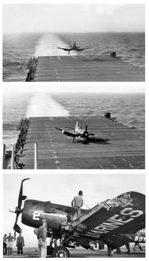
Second Lieutenant William Fitch bring an F4U Corsair aboard the USS Tarawa CVA-40, 19 May 1953; good landing, catches the threewire resulting in minimal damage to the aircraft. Incurring little damage, Fitch flew this F4U on a test flight off of the Tarawa ten days after the mishap.
