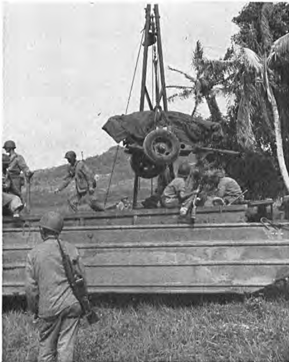
75MM PACK HOWITZER carried ashore in a DUKW is unloaded by an A-frame attached to another DUKW.
