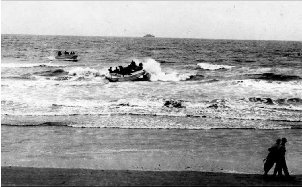
The exercises at New River included many Higgins boats. Lacking the bow ramp, these vessels were more difficult to exit than the later LCP. Here, troops struggle to hold the boat in the surf while others unload it. James Lipinski Collection, courtesy of 16th Infantry Regiment Association
