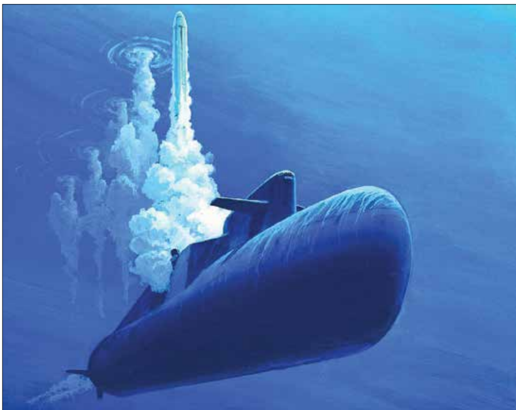
Edward L. Cooper, an artist working as a visual information specialist for the Defense Intelligence Agency, portrays a Soviet Delta III -class nuclear-powered ballistic missile submarine firing SS-N-18 Stingray missiles. The Delta III submarine was 155 meters long, had 16 missile firing tubes, and carried SS-N-18 nuclear missiles. Edward L. Cooper, Soviet Delta Submarine Firing SS-N-19 Missile , 1987. Lithograph. DIA Military Art Series: The Threat in the 1980s, Defense Intelligence Agency
