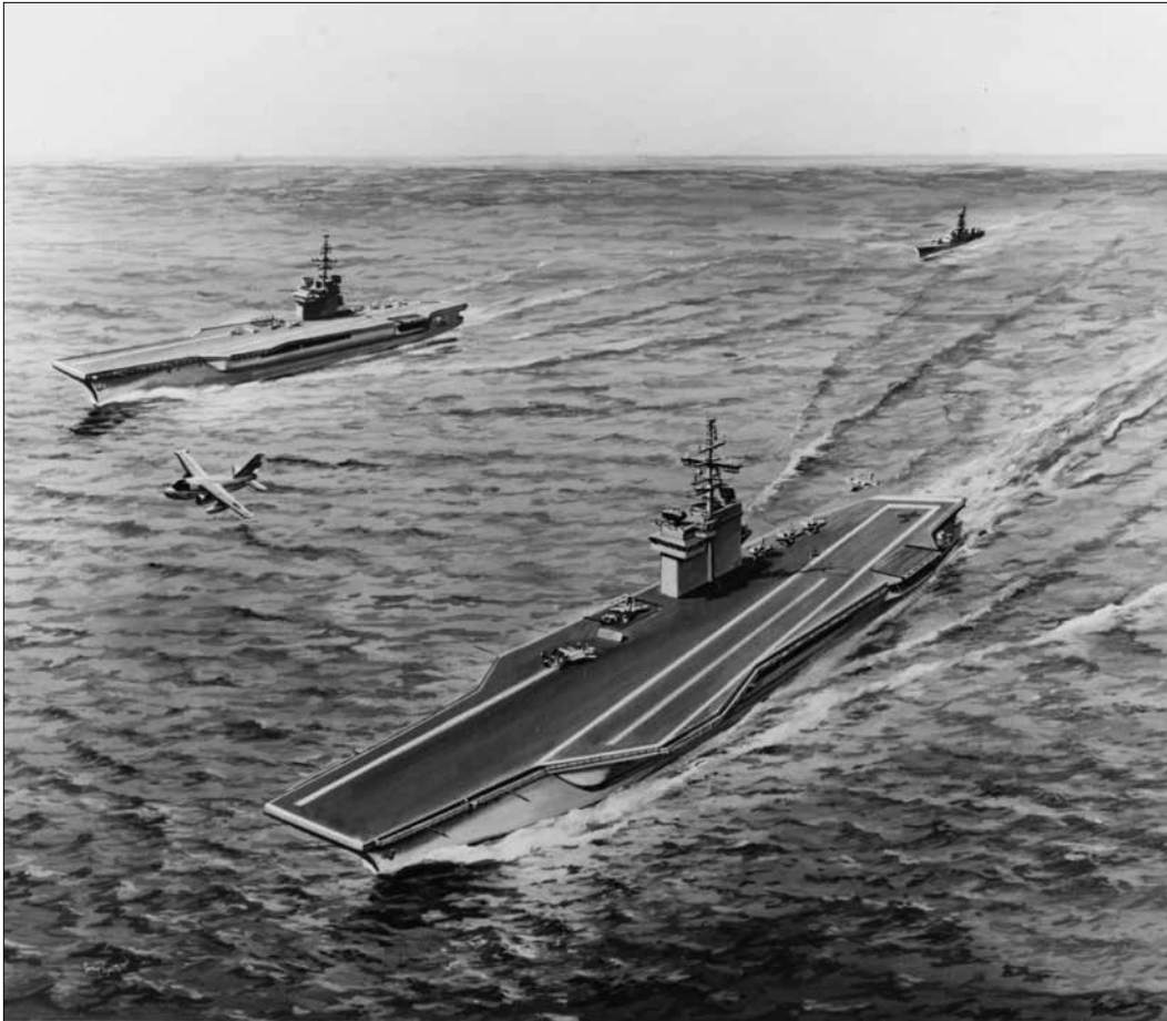
Artist's conception of the aircraft carrier proposed by the administration in 1978 for inclusion in the fiscal year 1980 Navy shipbuilding program. This 62,500-ton ship would have a length of 912 feet and an extreme width of 256 feet. It would be capable of operating all present and planned types of carrier aircraft. S. L. Morison, watercolor, 1978.
