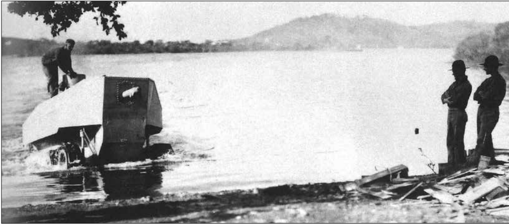
John W. Christie's amphibious tank lands on Culebra during the U.S. Marines' 1924 winter maneuvers. The experimental amphibious tractor began a long line of test vehicles that culminated in the landing vehicle, tracked (LVT).
