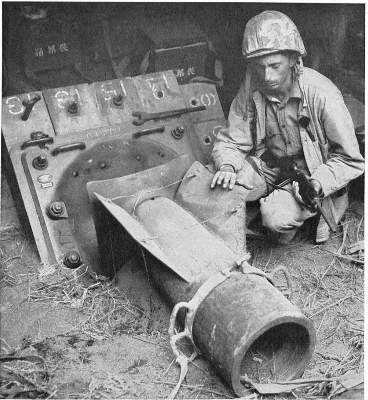
320MM SPIGOT MORTAR showing steel cylinder, base plate, and wooden platform.
