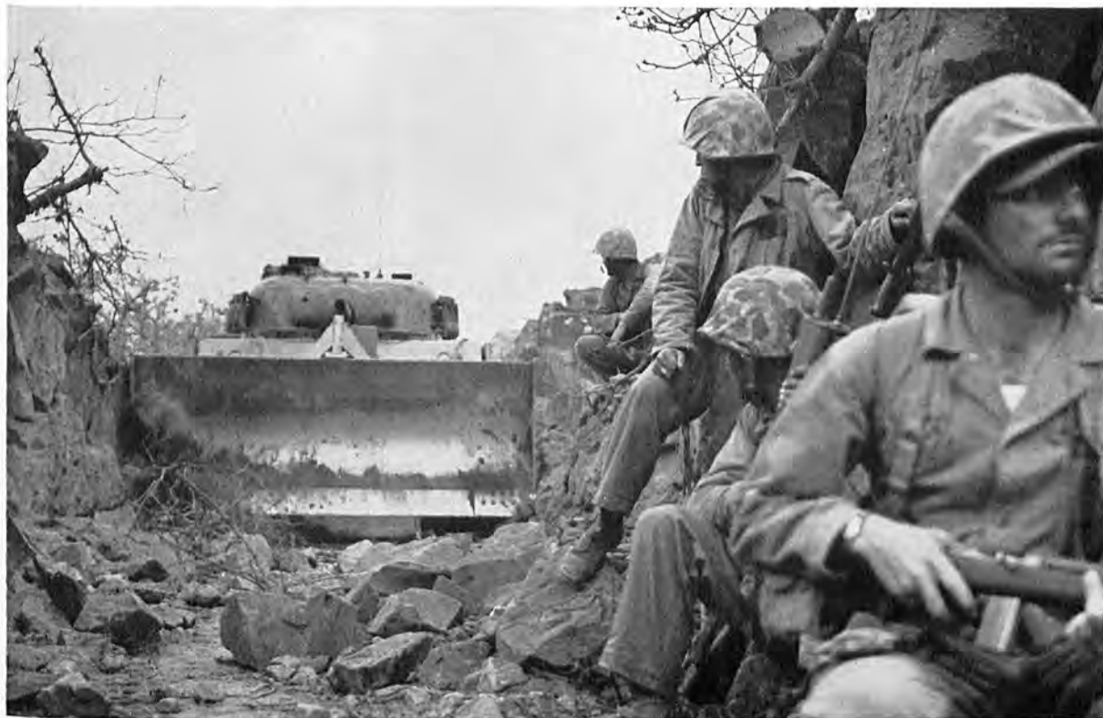
TANKDOZER clears route through rocky defile. Terrain such as this limited tank operations and dozers became an integral part of any tank-infantry team.
