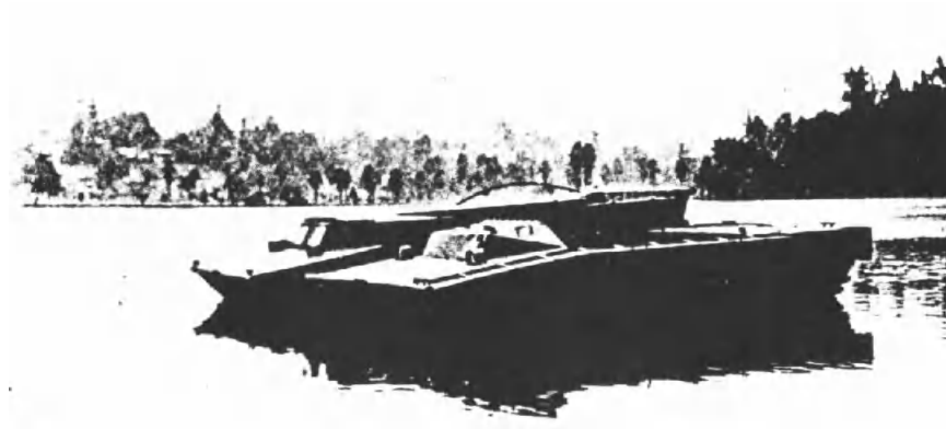
Figure 25. The LVT(4) and LVT(2) in a floating comparison. Note that the LVT(4) floats about one foot higher.
