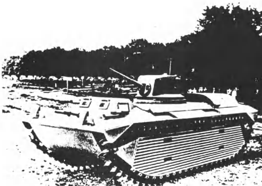
Figure 9. The Borg-Warner Model A with its tank turret and 37mm gun in place.
