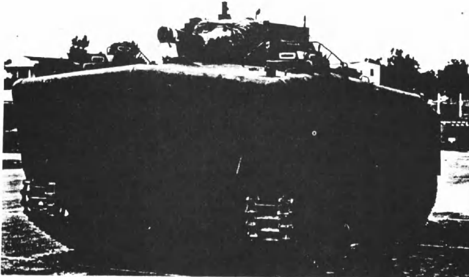
Figure 52. The LVT(H)6 with its powerful 105mm howitzer. This vehicle remains the only armored amtrac available for service, despite its age.
